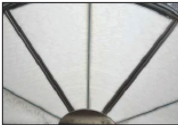
Figure 18 Embedded stiffener faces motor side.
