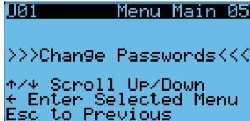
Technician Menu is password protected. Under the Technician Menu, the pressure sensor calibration can be adjusted between -99.9 and 99.9 psig total offset. Typically if a sensor is out of tolerance by more than 10.0%, it should be replaced. To adjust the calibration press the enter button to move the cursor to the desired field for adjustment. Pressure up or down to adjust as required and press enter to save the change.
