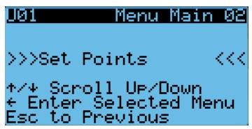
System Settings is the Set points menu. Set Point is the main set point control value that is trying to be maintained. The fans will increase and decrease speed trying to maintain this set point.
