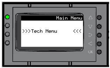
Enter a password of 9995 to enter and calibrate the pressure sensors under the technician's menu.
