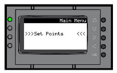
System Settings is the Set points menu. Set Point is the main set point control value that is trying to be maintained. The fans will increase and decrease speed trying to maintain this set point.
